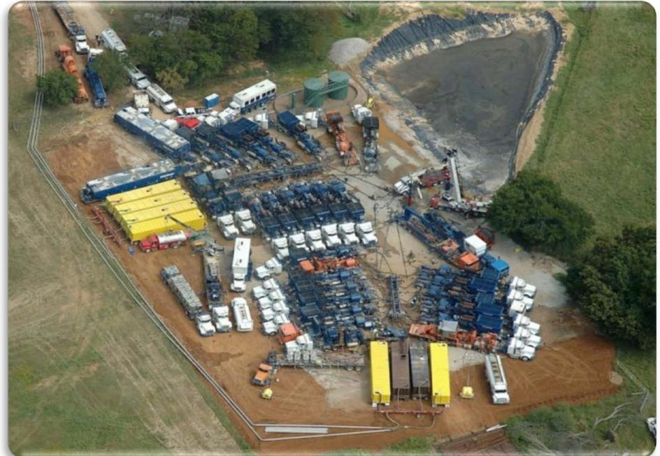
Dowell engineers use specialized equipment to perform high-injection-rate fracturing treatments on oil and gas wells.
