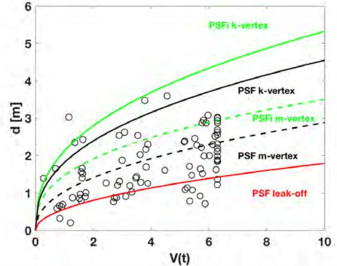
All events are located below the injection point and the fracture propagates downward. From the seismic cloud, only a partial penny-shaped fracture occur, whereby the error for small injection volumes is small.
