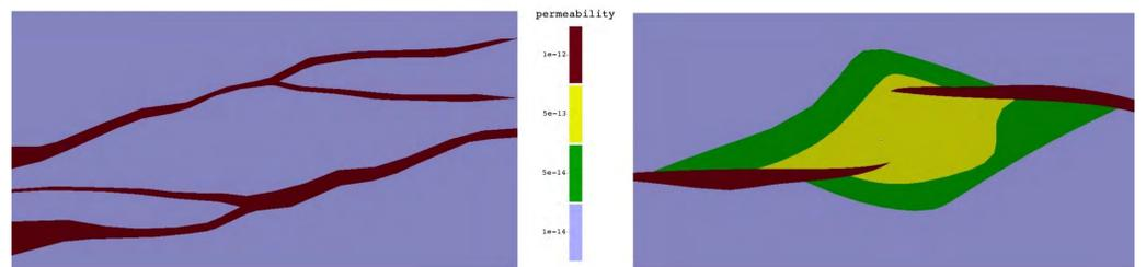
**Figure 1:** Geometry 1 (left cross-section) is aimed at showing the propagation of the dolomitization front through a porous matrix with two fracture zones of higher permeability. Geometry 2 (right cross-section) mimics a fault stepover with damaged matrix in the stepover zone. Both geometrical cross-sections vary slightly across the third dimension in an attempt to trigger non-uniform advancing chemical fronts.
