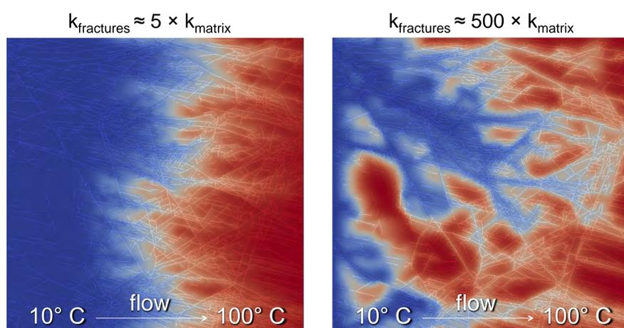
Fig. 2. Cold (10°C) water injection into a hot (100°C) fractured reservoir. Fracture permeability on the right figure is 100 times larger than the left (using CSMP++ with altered parameters from<sup>2</sup>).
