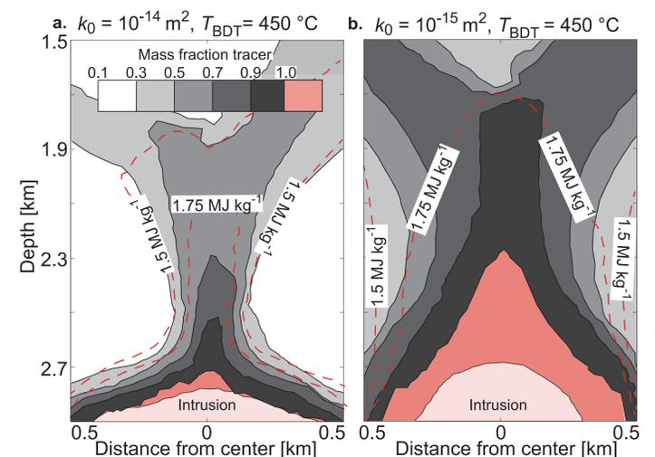
**Fig. 4: Colour scale indicates mixing (in terms of mass fraction) of fluid ascending out of the supercritical reservoir (mass fraction 1, red) and cooler liquid and/or vapour (grey tones).**
