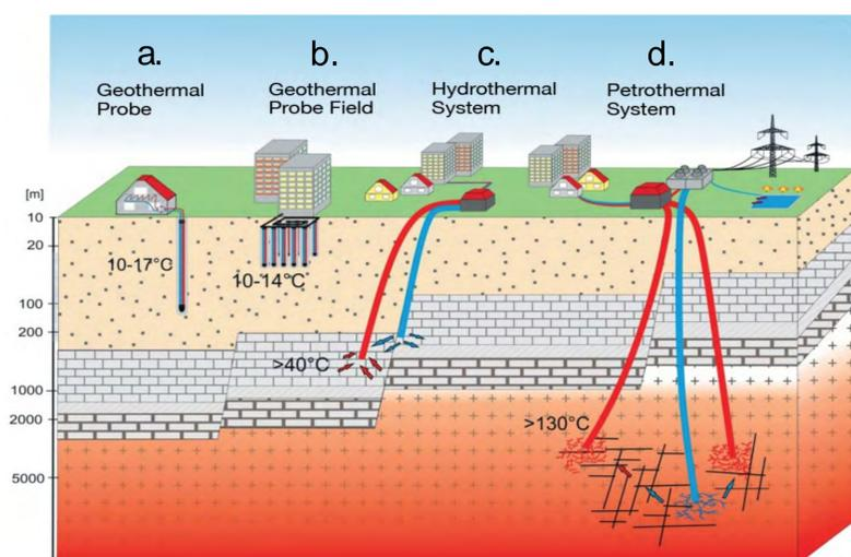
Fig. 1. Traditional geothermal techniques are shown in (a.), (b.), and (c.), while an EGS project is shown in (d.).<sup>1</sup>
