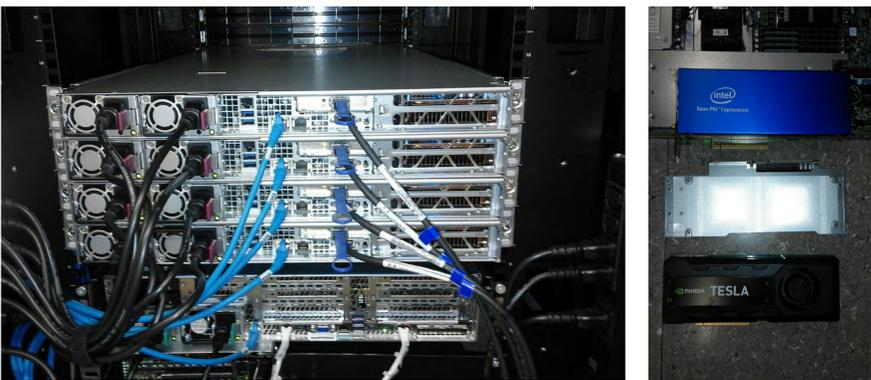
**Figure 1:** a) View of GPU/MIC cluster Thor recently installed at the University of Neuchâtel. The setup includes 4 computing nodes each equipped with two GPU Tesla 40K cards, one Intel Xeon Phi (MIC) coprocessor card, two 2 CPU 10 core Intel Xeon E5-2650, and Infiniband connection at 56 Gbits/s. The system includes about 1TB RAM and 20TB storage. This system, once proven, can be upgraded by adding additional nodes.
