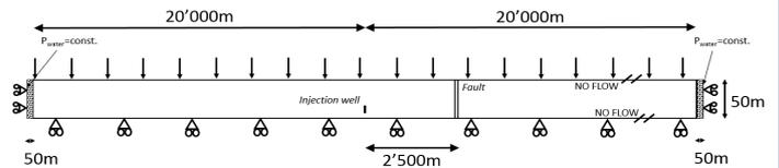
Figure 2. Schematic representation of the model geometry
