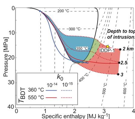
**Fig. 5 (left): The thermal structure of high-enthalpy geothermal systems. Pressure-enthalpy ascent paths are superimposed onto a phase diagram of water. The areas of potentially exploitable supercritical fluid, single-phase vapour, and two-phase fluid are shown in red, green, and blue, respectively. The measured reservoir temperature and enthalpy for the IDDP-1 well is shown with a yellow star.**
