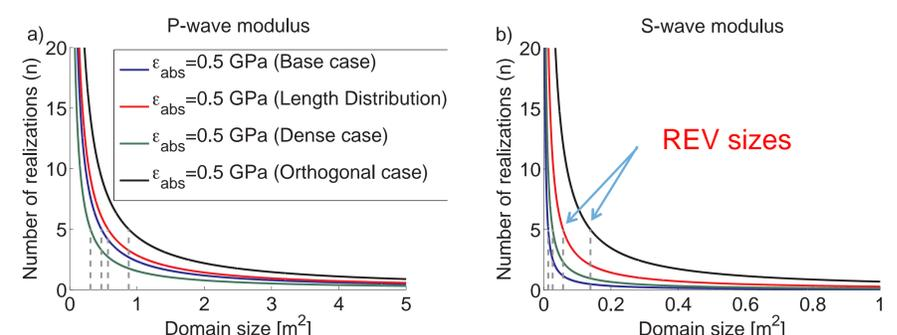
Figure 2: Number of realizations for an absolute error of 0.5 GPa of the upscaled a) P- and b) S-wave moduli as functions of the domain size at the lowest frequency. The dashed grey lines indicate the size of the REV for 5 realizations.
