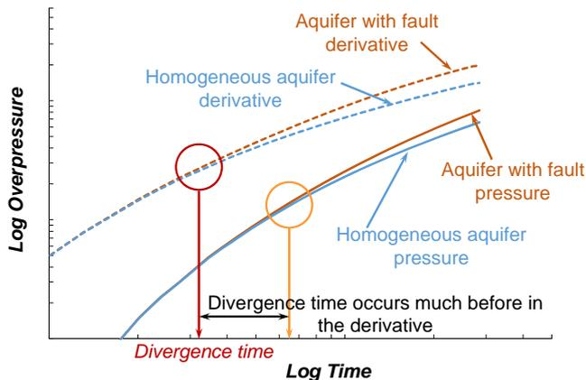
Figure 1. Diagnostic plots are a useful tool to anticipate to additional overpressure induced by the presence of undetected low permeability faults
