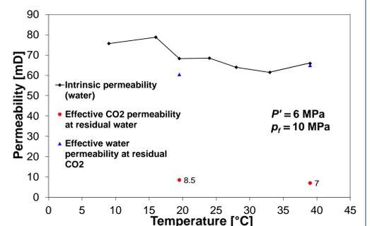
Fig. 5: Water and CO<sub>2</sub> permeability of water-saturated sandstone at different temperatures.
