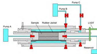
Figure : Experimental setup.
