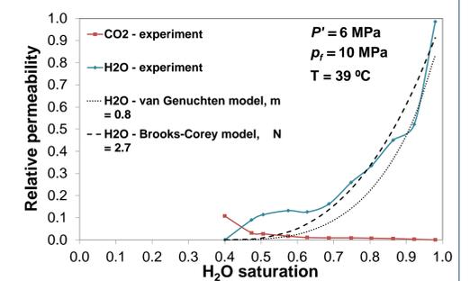
Fig. 7: Relative permeability of H<sub>2</sub>O and scCO<sub>2</sub> and fitting with different models.
