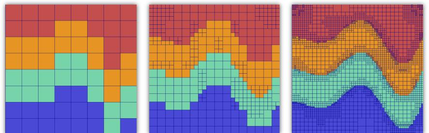
Fig 2. Adaptive mesh refinement based on the contrast of material properties of the geological setting.
