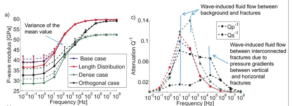
Figure 1: Mean value and variance for a) the P- and b) S-wave moduli as functions of frequency. The solid lines denote a domain size of 1.44 m<sup>2</sup> and the dashed lines of 0.09 m<sup>2</sup>. c) Corresponding attenuation of the P- and S-wave modulus (S=1.44 m<sup>2</sup>).
