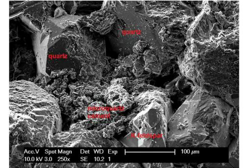
Fig. 4: Microphotograph of Berea sandstone.
