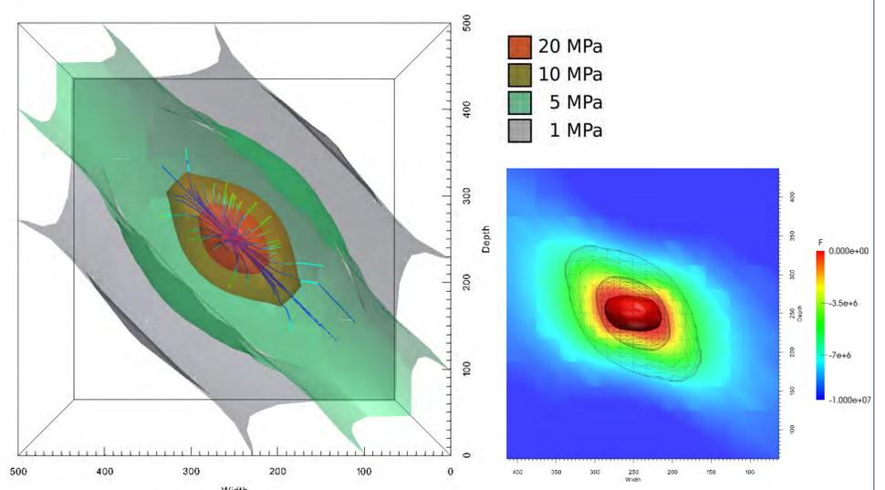
Fig 4. a) Fluid pressure isosurfaces and velocity streamlines for tracer particles inserted at the source. b) Plastic deformation zone envelope close to the 10MPa fluid pressure isosurface
