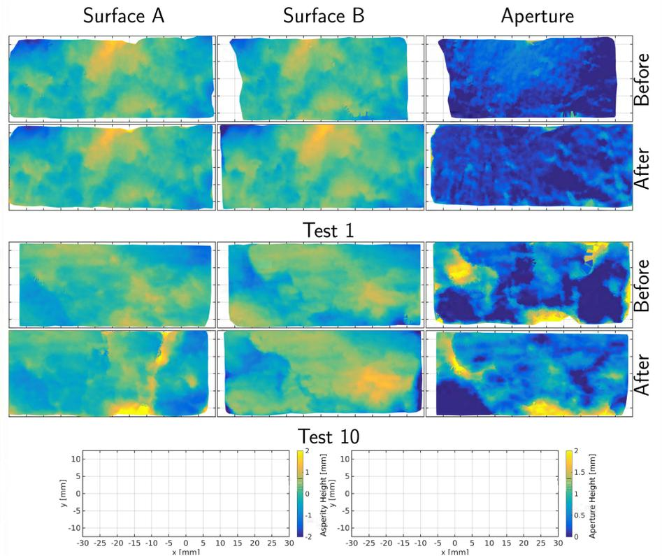
Photogrammetric scans of fracture surfaces before (top) and after (bottom) testing allow investigation of roughness, damage and strength between surfaces and apertures.
