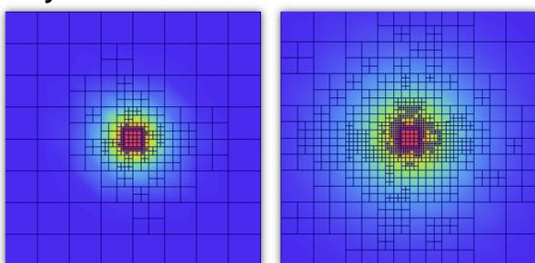
Fig 1. Adaptive mesh refinement for a diffusion process based on the gradient of the fluid pressure
