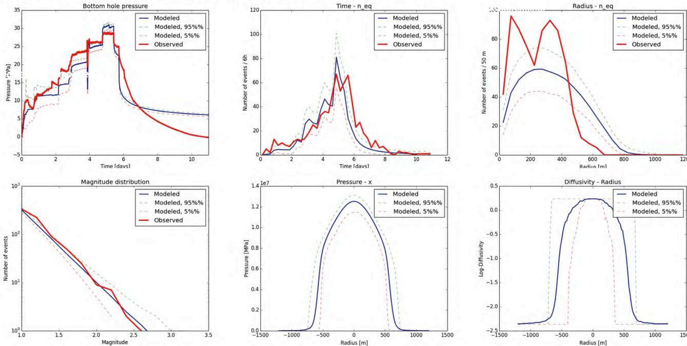
Two-way coupled simulation implemented in Python using the FiPy software package for the non-linear diffusion simulation and MPI4Py for parallelisation. With the MPI parallelisation, the simulation scales perfectly up to 1000 CPUs (number of forward runs).
