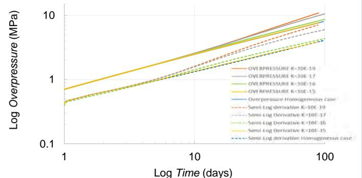
Figure 3. Sensitivity of overpressure to the permeability of the fault, measured at a distance from the injection well equal to two times the aquifer thickness (towards the fault)
