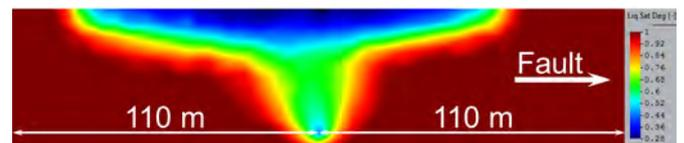
Figure 4. CO<sub>2</sub> plume shape affected by a low permeability fault
