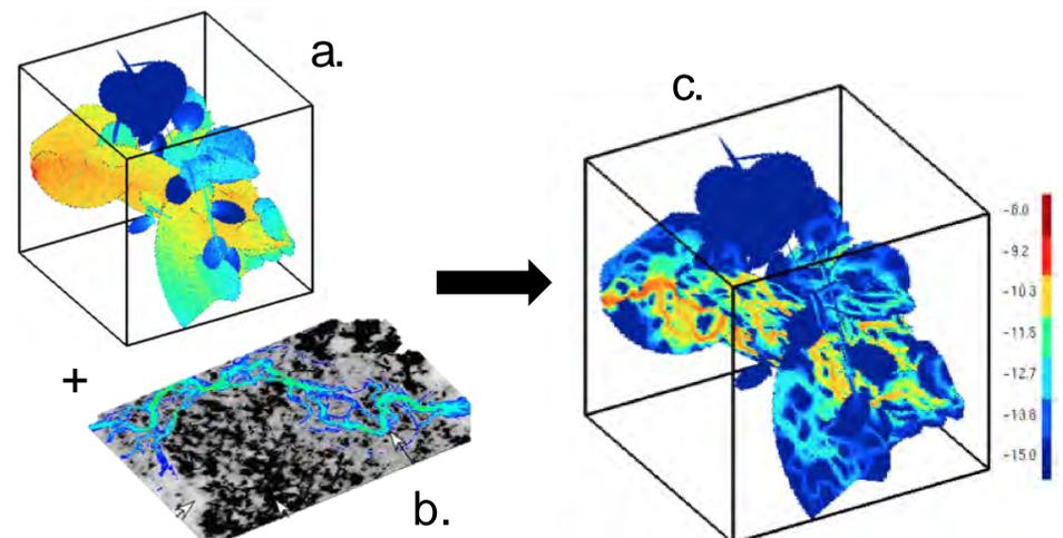
Fig. 3. The combination of flow in a fracture network (a.)<sup>3</sup> and flow in a heterogeneous fracture (b.)<sup>4</sup> results in a highly channelized flow (c.)<sup>3</sup> with poor reservoir sweep efficiency. Scale on right displays logarithm of mean flow value
