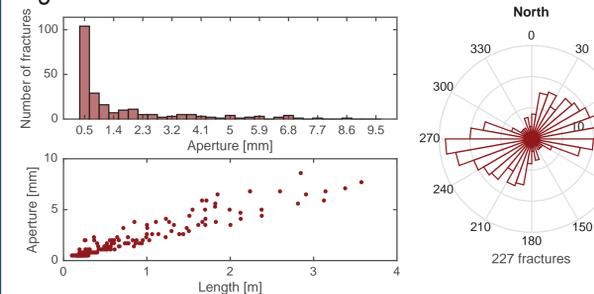
Fig 6: Distribution of aperture (top left), orientation (right), and length (bottom left) of the fractures shown in the model in Fig (7, left).
