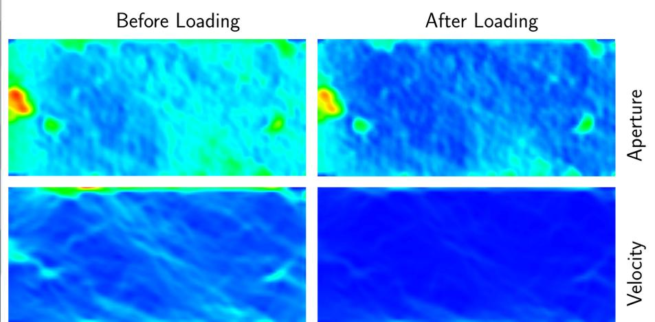
Hydro-Mechanically coupled fluid flow during normal loading in the experiments is simulated with the GEOS framework developed at LLNL.
