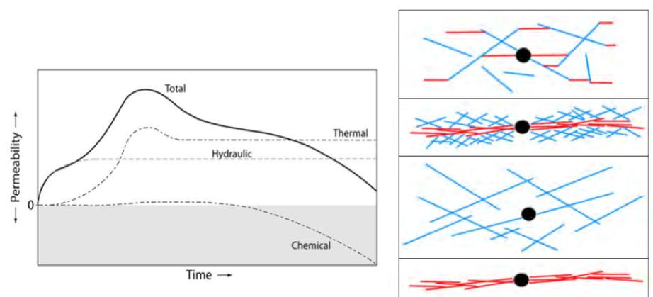
Fig. 3. (left) Relative time scales of the processes effects on fracture permeability throughout reservoir's life.<sup>5</sup> (right) Various geomechanical possibilities of fracture network growth around a well during stimulation.<sup>6</sup> Red lines represent new fractures due to tensile failure; blue lines represent preexisting fractures enlarged due to shear slippage.
