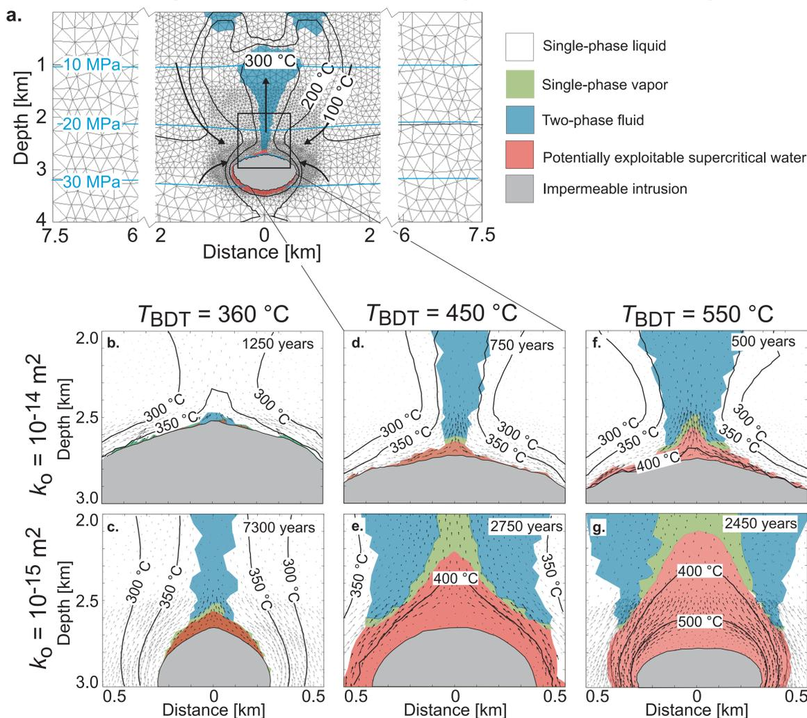
**Fig. 3: a. Typical large-scale thermal structure of a simulated geothermal system b-g. Snapshots of the area near the top of the intrusion (black box in a.), under different conditions of host rock permeability ( $k_0$ ) and brittle-ductile transition temperature ( $T_{BDT}$ ).**
