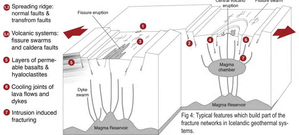
Fig 4: Typical features which build part of the fracture networks in Icelandic geothermal systems.
