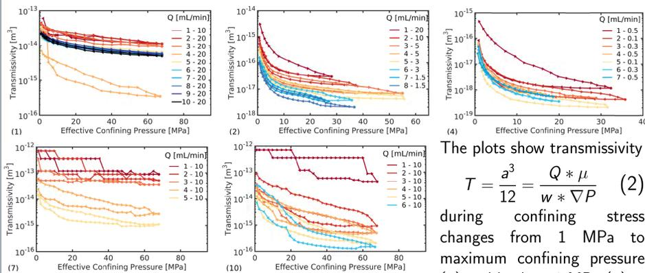
The plots show transmissivity  $T = \frac{a^3}{12} = \frac{Q * \mu}{w * \nabla P}$  (2) during confining stress changes from 1 MPa to maximum confining pressure (▷) and back to 1 MPa (◁).
