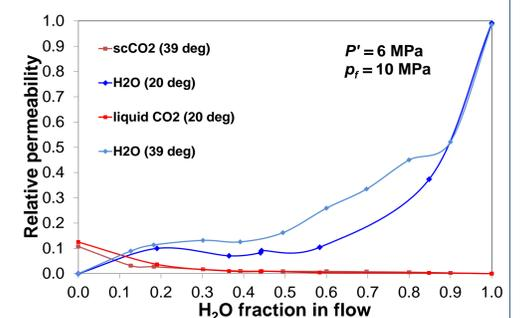
Fig. 6: Relative permeability of H<sub>2</sub>O and CO<sub>2</sub> at 20°C and 39°C vs H<sub>2</sub>O fraction in flow.
