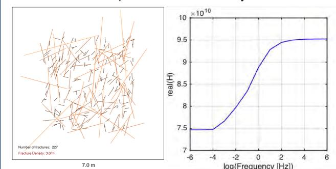
Fig 7: Model of the fracture network (left) and the corresponding P-wave modulus  $H$  resulting from the oscillatory compressibility test (right).
