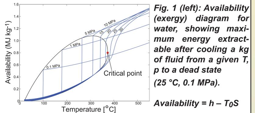
**Fig. 1 (left): Availability (exergy) diagram for water, showing maximum energy extractable after cooling a kg of fluid from a given  $T, p$  to a dead state (25 °C, 0.1 MPa).**
