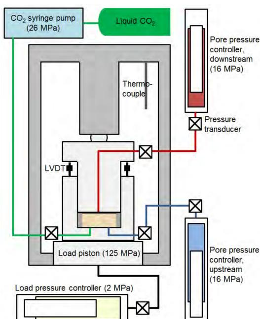
Fig. 3: Experimental setup: oedometric cell.
