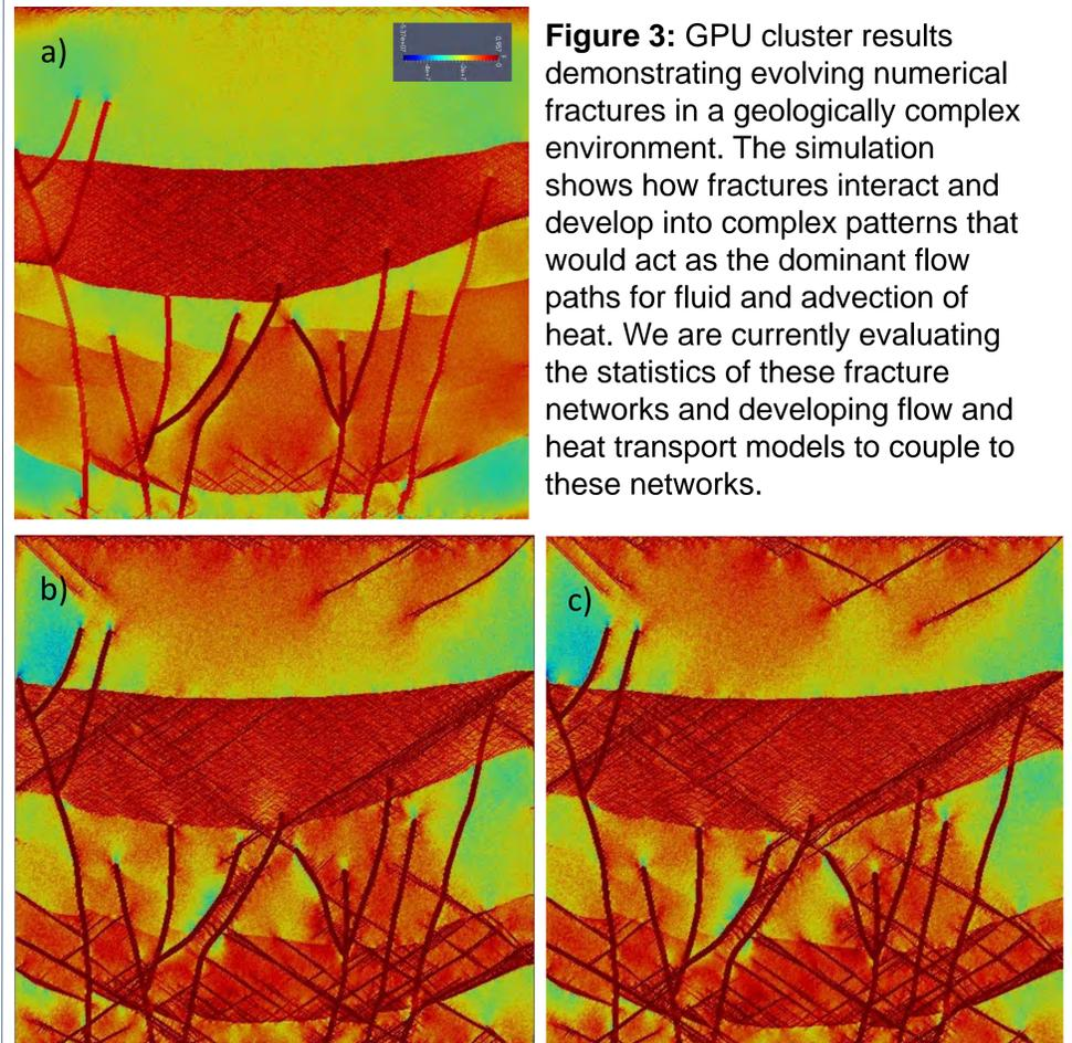
**Figure 3:** GPU cluster results demonstrating evolving numerical fractures in a geologically complex environment. The simulation shows how fractures interact and develop into complex patterns that would act as the dominant flow paths for fluid and advection of heat. We are currently evaluating the statistics of these fracture networks and developing flow and heat transport models to couple to these networks.
