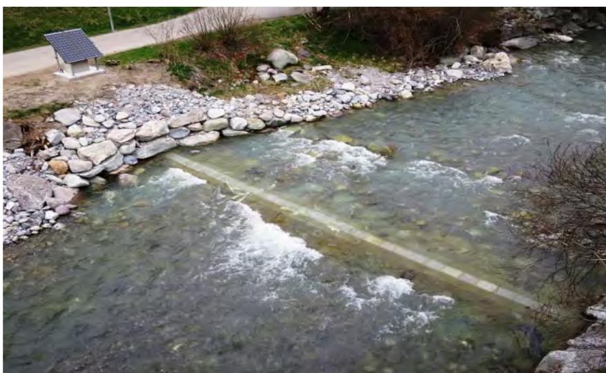
Fig. 1: New geophone measuring station in the Albula River in Tiefencastel
