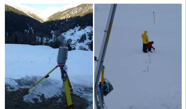
Figure 6: Terrestrial laser scanning (left) and manual snow observations (right) during snow making test
