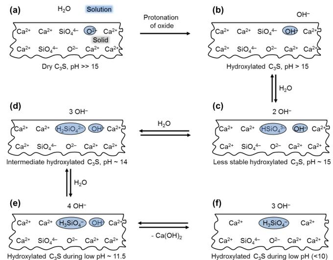
Figure 3. Schematic of different possible steps of dissolution of  $C_3S$  which involves hydration of superficial oxide ions as well as formation of silanol groups.
