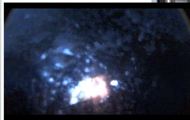
Oxygen-ethanol flame burning in water at 26 MPa
