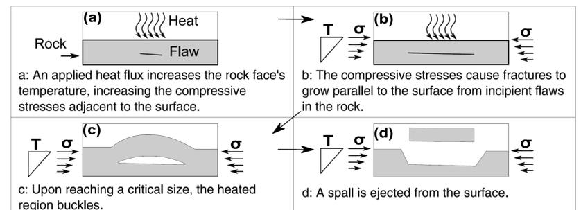
Fig. 2: Spallation model by Preston and White[1], modified from Walsh and Lomov [4]
