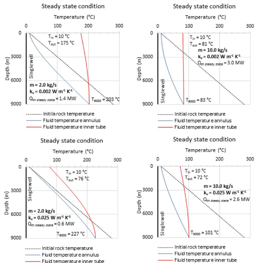
The results are shown for two mass flow rates  $m$  of the circulating fluid and for two different thermal conductivities  $k_v$  of the double-wall pipe. The thermal power produced at steady state  $Q_{th}$  is given in the graphs above.
