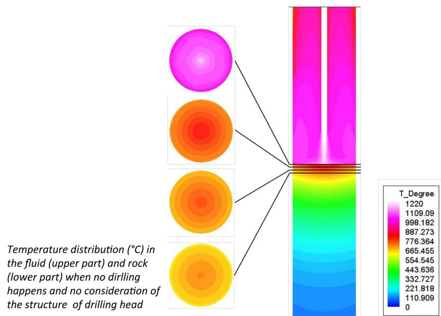
Temperature distribution (°C) in the fluid (upper part) and rock (lower part) when no drilling happens and no consideration of the structure of drilling head
