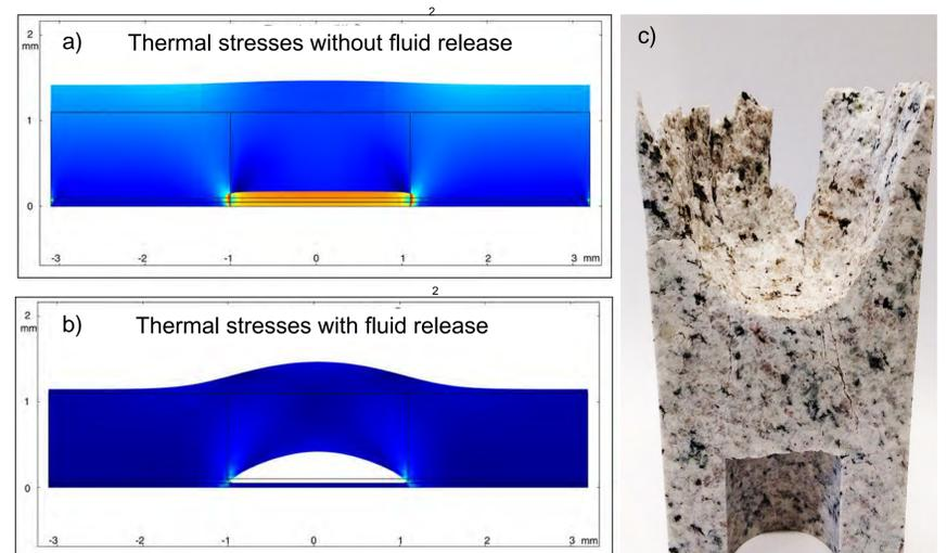
Fig. 4: a) Differential expansion of quartz and biotite. b) Same model with water replacing part of the biotite c) rock sample after the spallation experiment
