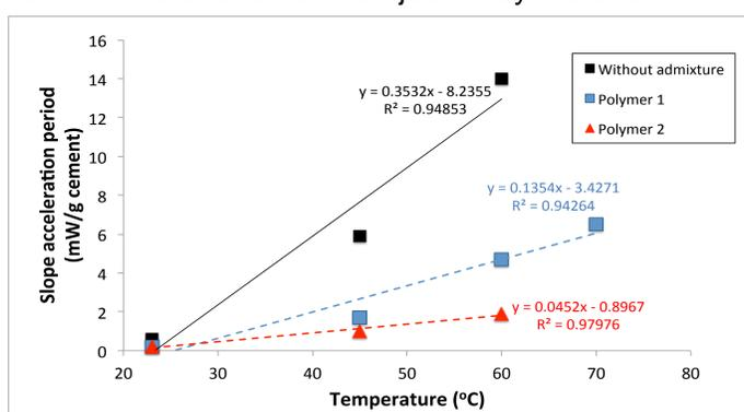
Figure 2. Slope of the acceleration period of cement pastes at different temperatures
