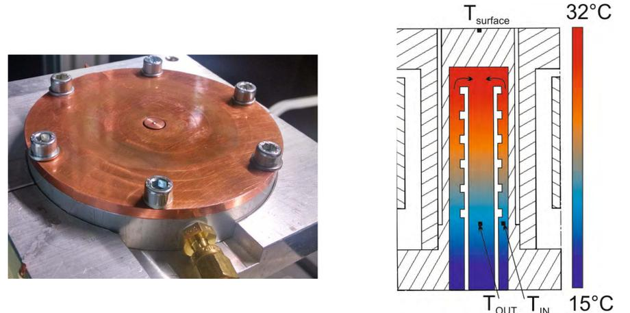
Fig. 4 Calorimeter – heat flux sensor Fig. 5 Cross section of the sensor
