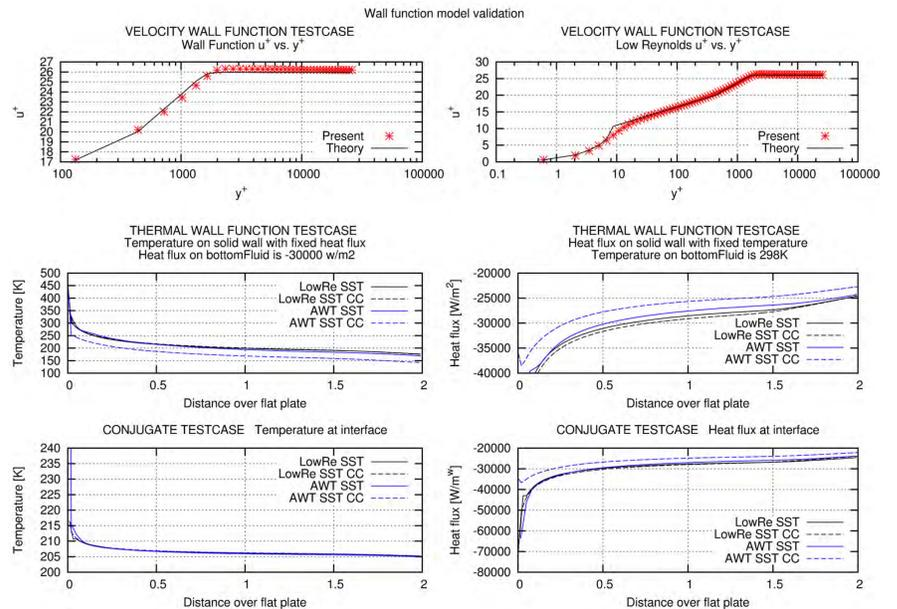
Fig. 2: Flat plate test case with and without conjugate heat transfer. The results labeled «CC» were obtained using a commercial code. The «AWT» label indicates the use of wall functions.
