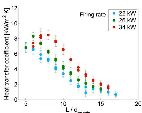
Fig. 3 Heat transfer study from the impinging flame jet to a heat flux sensor
