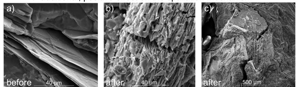
Fig. 3: SEM pictures: a) before spallation, b),c) after spallation
