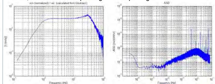
The passing band of the sensing loop can be modified, either to reduce the lower corner frequency, e.g. to 50mHz (already tested), or to increase the upper corner frequency, to e.g. 1kHz (to be tested).
