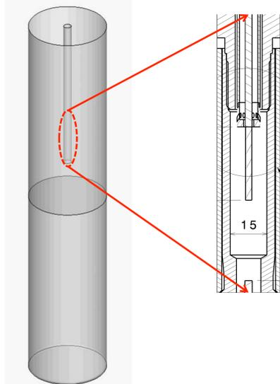
Schematic diagram of the simulation domain: combustion chamber and rock
