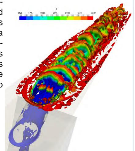
Fig. 4: Turbulent structures of a cooling jet in crossflow at low blowing rate
