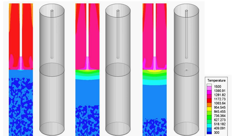
Temperature distribution (K) and drilling process at different time: 0s, 20s, 40s, 60s, 80s, 100s
