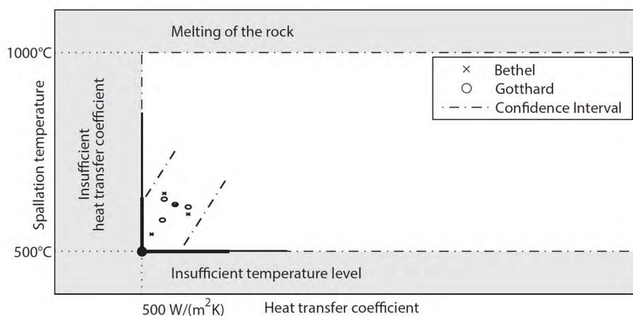
Fig. 1: Applicable operating conditions for thermal spallation drilling with experimental measurements for the determination of the minimal applicable boundary conditions
