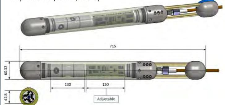
The sensor cabinet can be adapted to classic geophone sensors, or to the new spherical sensor (larger diameter required). With this housing design, thermal simulations are done to determine heat flow from the electronics cabinet to the outside.
