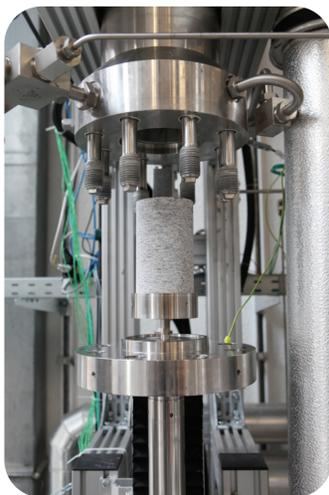
Fig. 2 a) High pressure drilling setup
