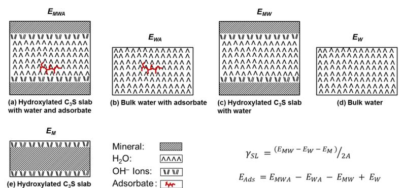
Figure 4. Schematic of the calculations of solid-liquid interfacial energy  $\gamma_{SL}$  and adsorption energy  $E_{Ads}$  using molecular dynamics simulations.
