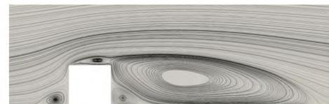
Fig. 3: Averaged streamlines behind turbulator
