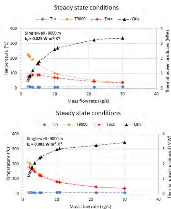
The two summarizing graphs on the left show the inlet temperature at the ground surface  $T_{in}$  (blue), the temperature of the circulating fluid at the base  $T_{9000}$  (orange), the outlet temperature at the surface  $T_{out}$  (red) and thermal power produced  $Q_{th}$  (black).
