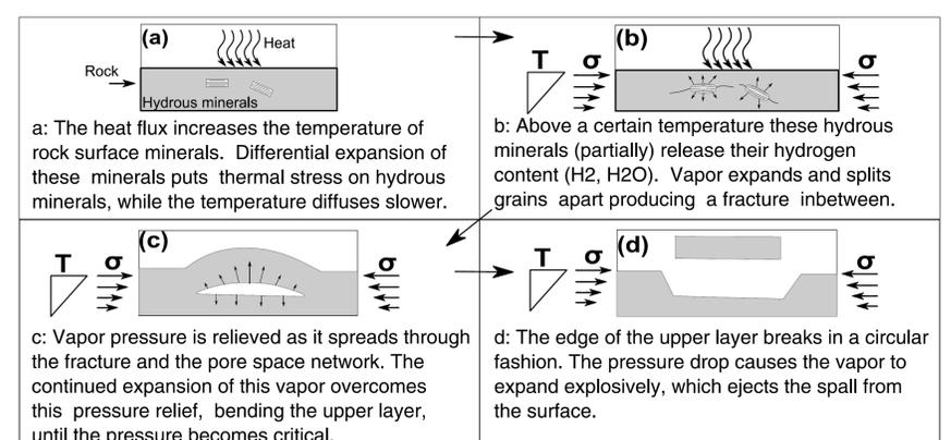
Fig. 5: Proposed additional thermal spallation mechanism (modified from Walsh and Lomov [4])
