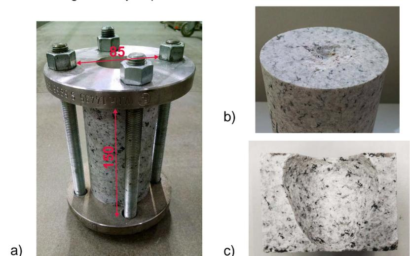
Fig. 6 a) compressed rock sample, b) results of spallation without compression b) with compression
