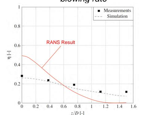
Fig. 6: Lateral cooling effectiveness of jet in crossflow
