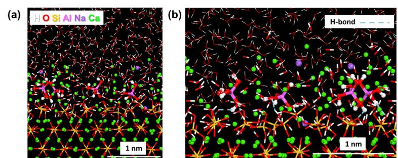
Figure 5. Interactions of aluminate ions with hyd.  $C_3S$  (a) Hyd.  $C_3S$  (formation of  $SiO(OH)_3^{1-} + H_2O + NaAl(OH)_4$ ), (b) Formation of hydrogen bonds between  $Si-O \cdots HO-Al$  or  $Si-OH \cdots O-Al$ .
