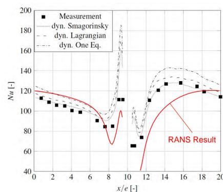
Fig. 5: Nusselt number distribution over turbulator for different LES models
