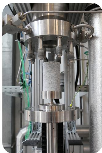
Fig. 2 a) High pressure drilling setup
