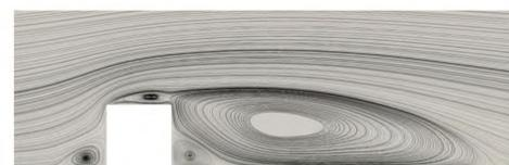
Fig. 3: Averaged streamlines behind turbulator
