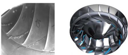
**Problem:** Formation of cavitation vortices in the inter-blade channels (inter-blade vortices) with unknown draft tube flow interaction and erosive potential.
