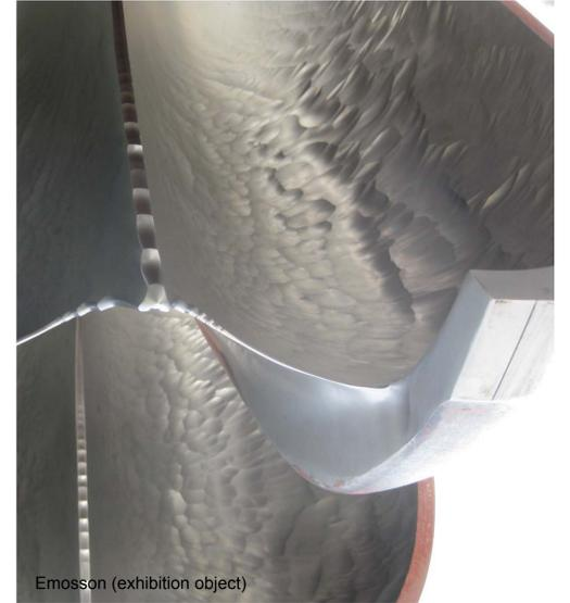
Fig. 2: Runner of Pelton turbine with abrasion damages
