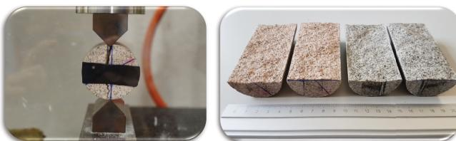
Fig. 1 Left: Brazilian induced fracture and Right: comparison of thermally shocked (left) and not shocked (right) samples.
