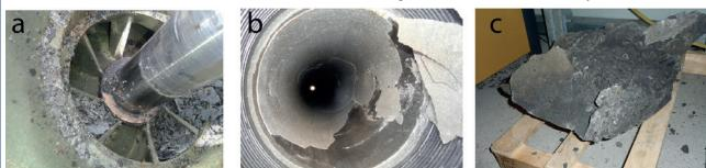
Fig. 2: Scales formed along (a) the pump, (b) the riser pipe, and (c) in installations of the geothermal plant at the surface.
