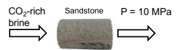
Fig.1 Sketch of the model with constant flow rate at the inlet and constant pressure at the outlet.
