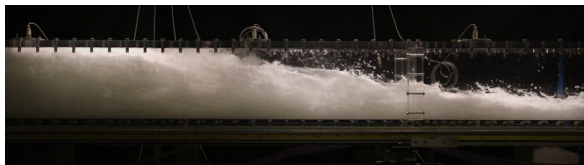
Fig. 2: A slug photographed in the hydraulic scale model. Flow direction from left to right.
