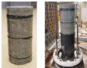
Figure 3: Fiber optic instrumented samples.
