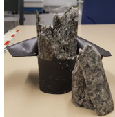
Figure 1b: Tested sample under 200 MPa and 200°C.
