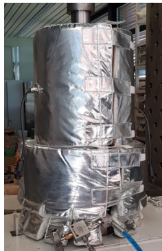
Figure 2: High PT triaxial device with heating jacket.
