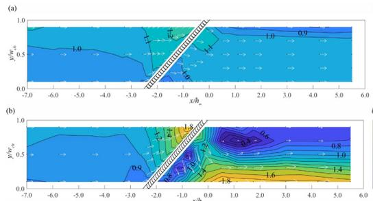
Fig. 4: Measured flow field of  $U/U_0$  at MCR configuration  $\alpha = 30^\circ$ ,  $s = 50$  mm (a)  $\beta = 45^\circ$  and (b)  $\beta = 90^\circ$ .
